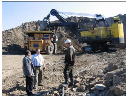
One of the original P&H 2300XP shovels placed into service in the Kuznetsk coal basin in Western Siberia during the 1980s (top photo); one of several original P&H 2800XPs that continue to provide productive service in the Kuzbass (center photo); a modern-era P&H 2800XPB loads a Belaz haul truck in a Kuzbass coal mine (lower photo).
