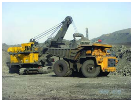
One of the original P&H 2300XP shovels placed into service in the Kuznetsk coal basin in Western Siberia during the 1980s (top photo); one of several original P&H 2800XPs that continue to provide productive service in the Kuzbass (center photo); a modern-era P&H 2800XPB loads a Belaz haul truck in a Kuzbass coal mine (lower photo).
